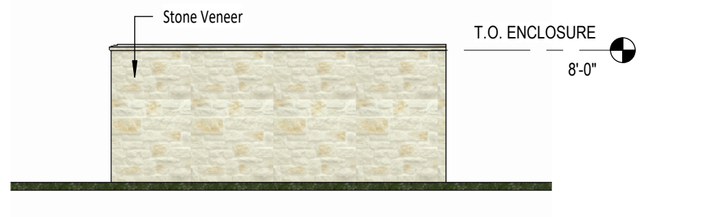
C1 Dumpster Enclosure - Side G3.00 1/8" = 1'-0"
